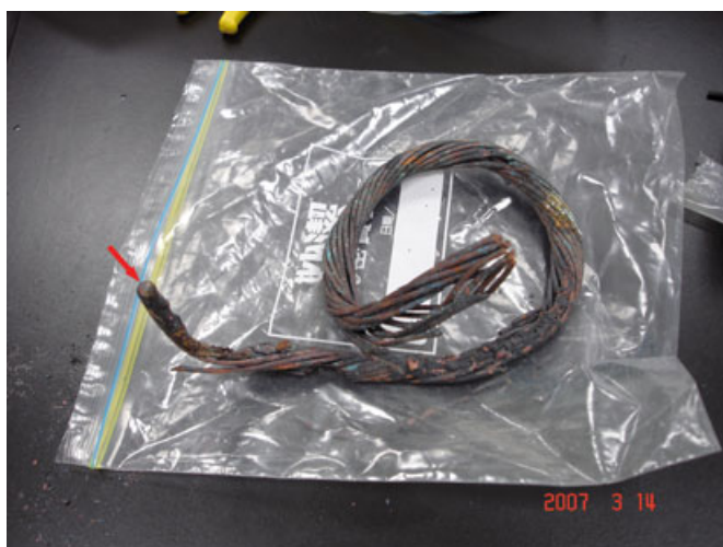
FIG. 2—View of cable with bead at the end (arrow indicates), the cross-section of the bead was used for further metallographic examinations.
