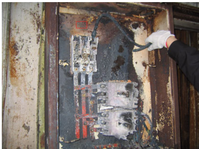
FIG. 1—Fire damage inside switchboard. The rectangle region of the steel plate was removed for metallographic analysis.
